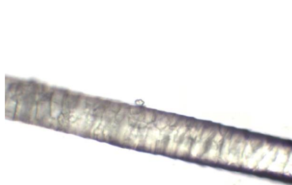
Fig.4. Microscopic image of washed wool fiber (30% lye/ 20x magnification degree)
